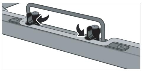
Once the bag's frame is in place, rotate the locking tabs (Part B) 90 degrees to lock the frame in place. Repeat on both sides.
