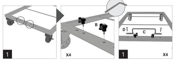
Install the 4 locking tabs (Part B) into the inner set of holes on both sides of the frame. Tighten with the Allen Wrench (Part F). Repeat on both sides.
