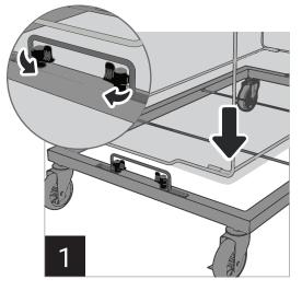
Make sure the locking tabs (Part B) are rotated in and pointed towards each other. Lower the bag onto the base with the bag's bottom frame on the outside of the base handle.
