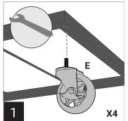
Install the four bottom castors (Part E). Use the wrench (Part G) to tighten.
