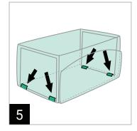
Secure inner frames with the four velcro straps in each corner.
