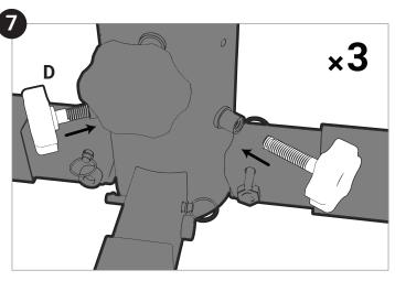
**OPTIONAL:** ADD LOWER KNOBS IF ADDITIONAL STABILIZATION IS NEEDED.
